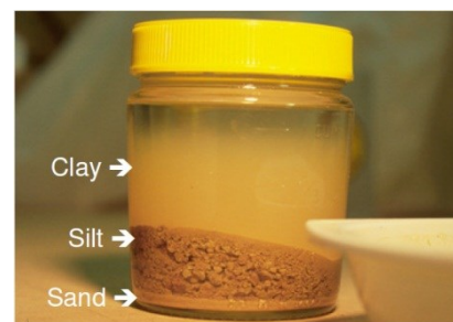
Particle Size – Turbidity vs Sediment
